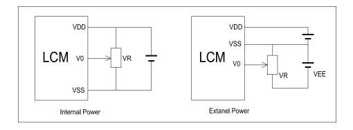
V<sub>DD</sub>-V₀: LCD Driving voltage VR: 10k~20k
